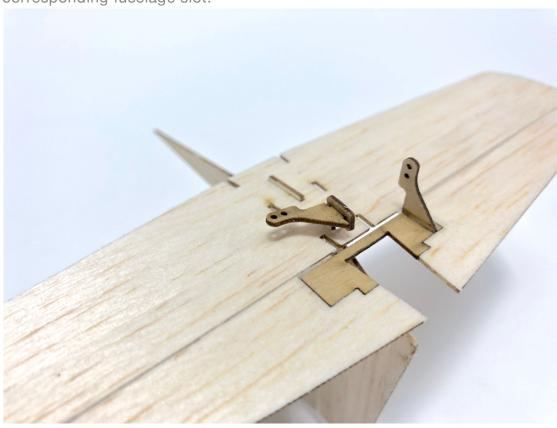
39. The rudder control horn must be installed on the side of the corresponding fuselage slot.
