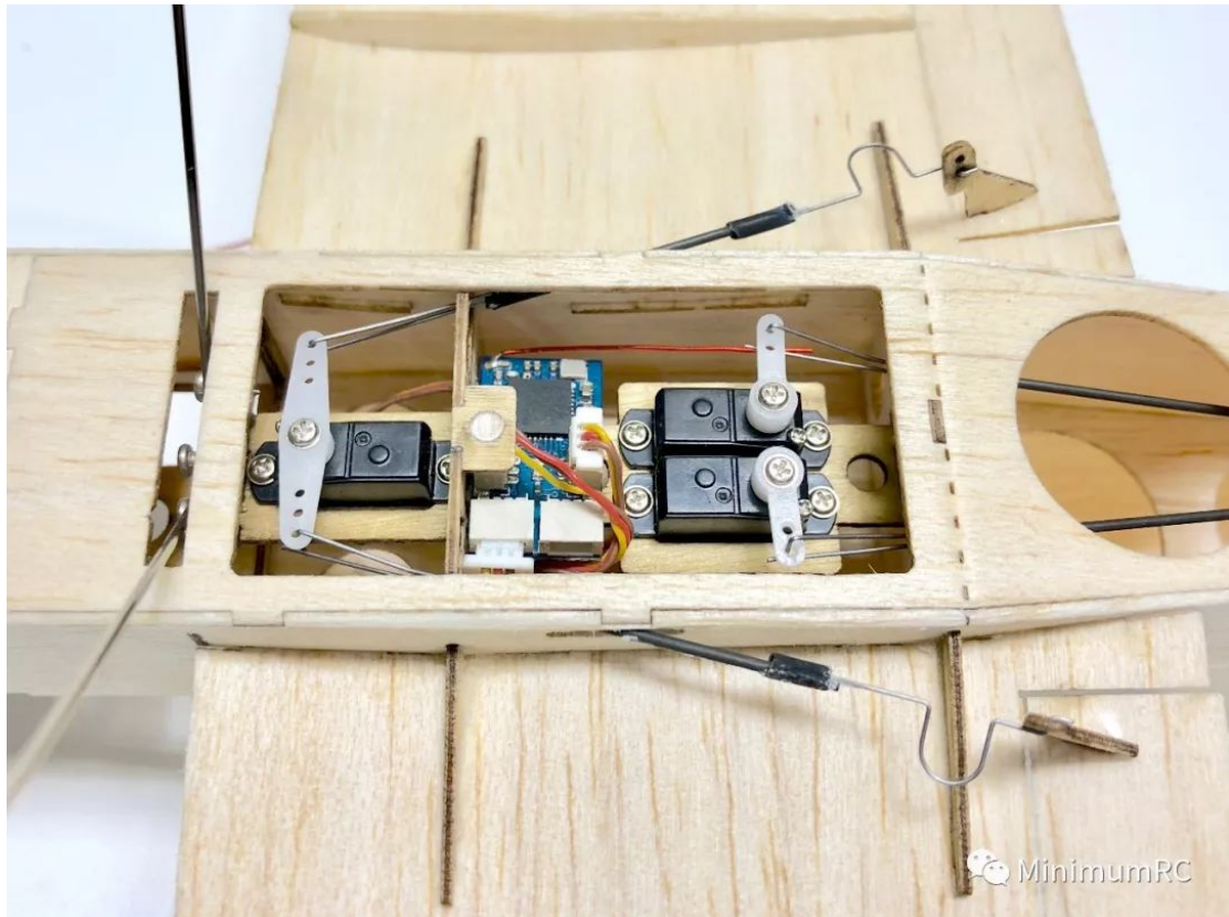
57. Installation of the receiver.
