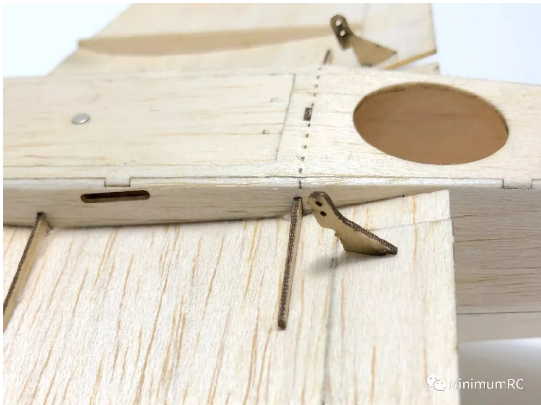
45. Installation of the control horns.
