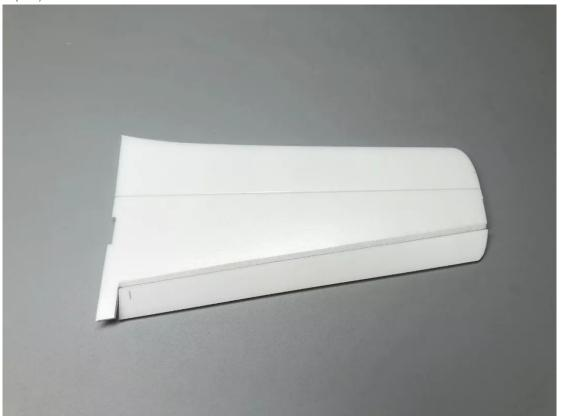
Sticking transparent tape on both sides to enhance the torsional rigidity of aileron
