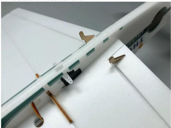
15. Connect the pushrod clips with heat shrinkable tube and fix them with glue.
