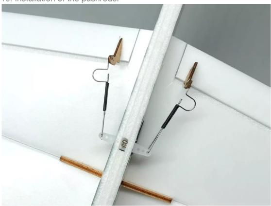
17. Installation of the control horns.
