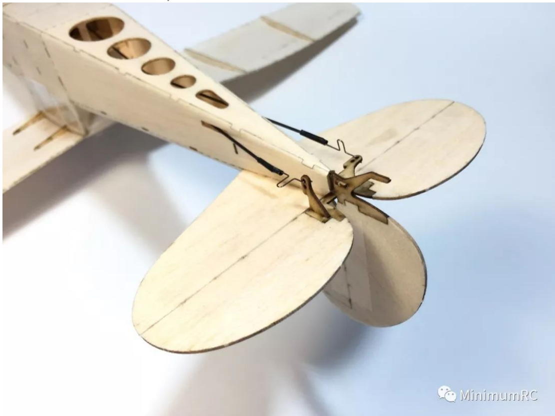
63. Installation of the pushrods.
