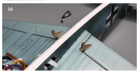
15. Glue the elevator & rudder control horns.
