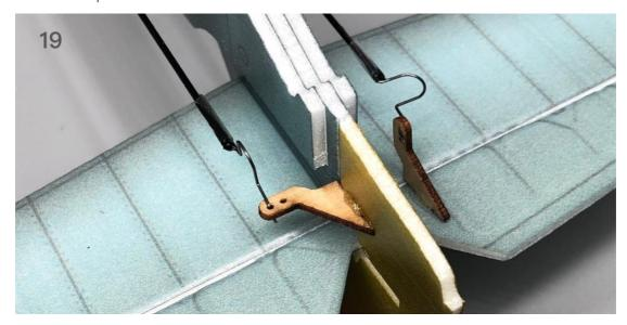
20. Use heat-shrinkable tube to connect steel wire clips for ailerons.
