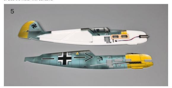
6. Glue both sides of fuselage together.
